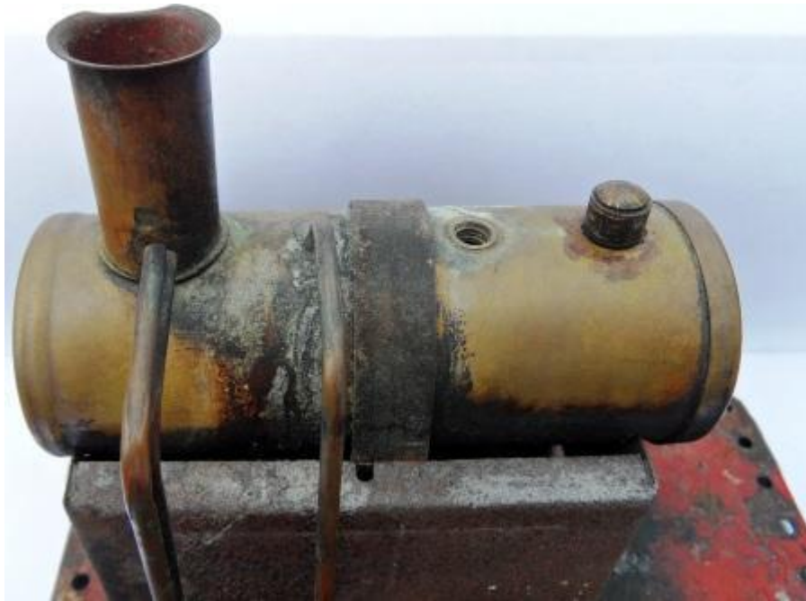
Plenty of rust, dented chimney.
