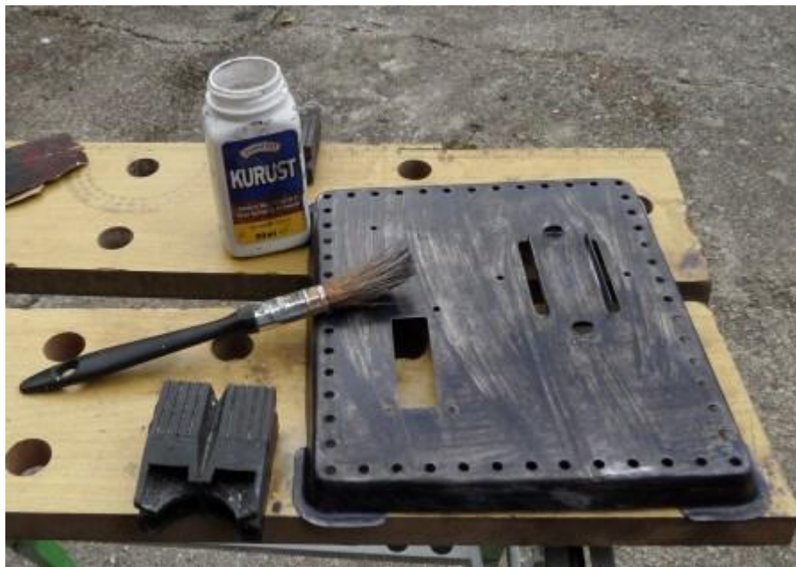
A generous helping of rust treatment
